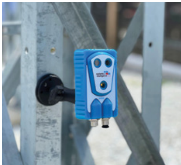
Figure 4. IoT sensors used for visual and thermal asset monitoring.
