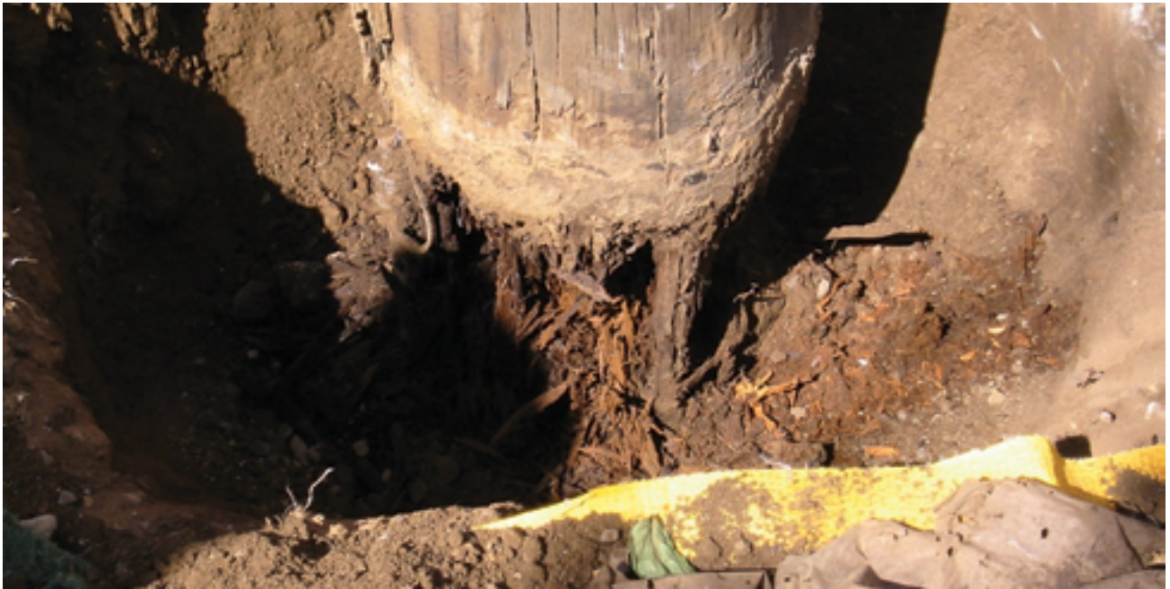
Shows the decay pattern of a thick sapwood pole because these poles decay from the outside-in Credit: Osmose Utilities Services
