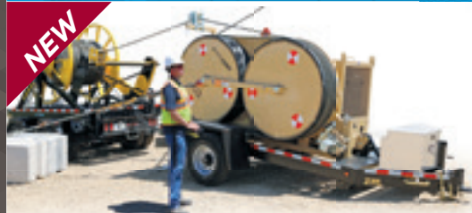
PT1250 11,240 lb. Single Rope or Conductor Puller-Tensioner
