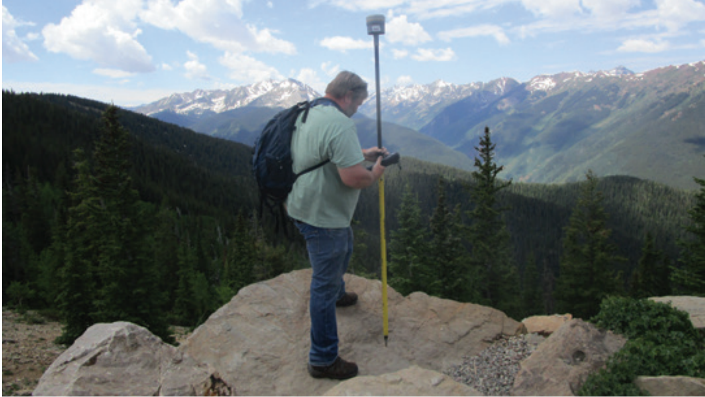
Far removed from the Nebraska plains, Kenna uses RTX for a real-time survey in the Colorado mountains. Satellite-delivered correction data ensures accurate results anywhere on Earth.
