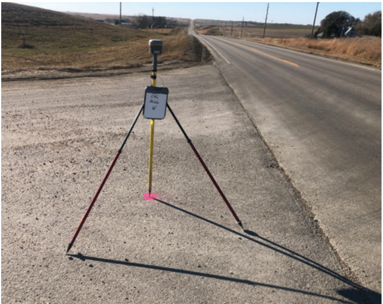
GNSS receiver uses RTX to produce precise position data. RTX enabled efficient real-time measurement without need for base stations or cellular connections.
