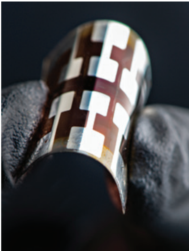
A flexible all-perovskite tandem solar cell. Photo by Dennis Schroeder / NREL.
