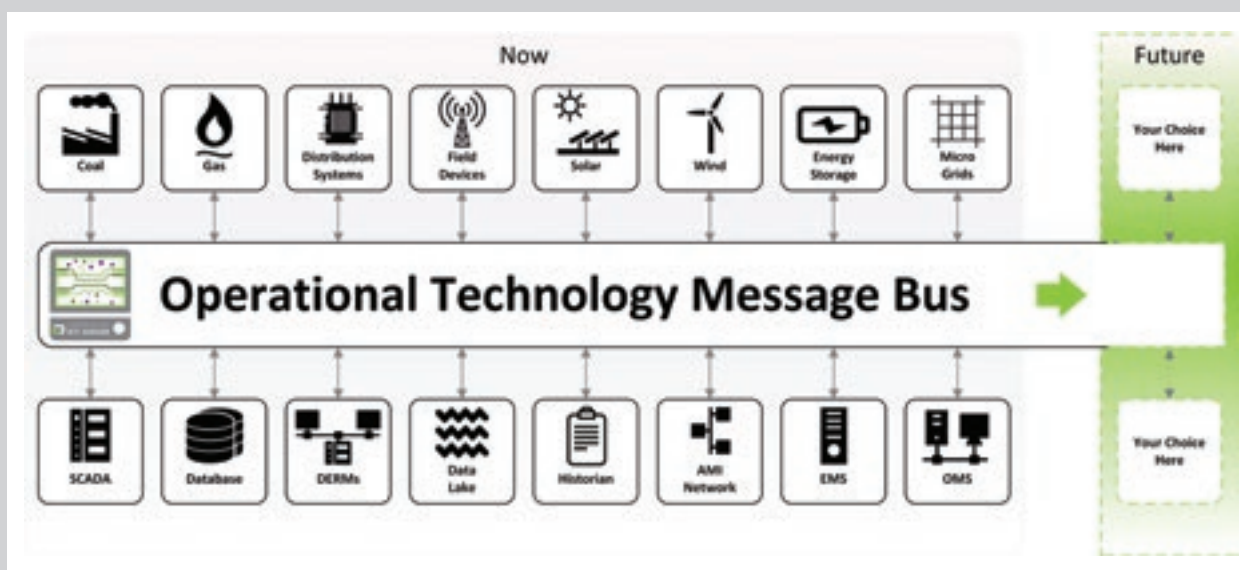
Figure 3. An OTMB architectural pattern allows for integration of all legacy, modern and future devices and systems.
