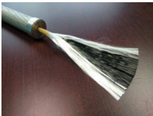
Carbon and glass fiber ACCC conductor core uses over 600,000 individual carbon fibers
