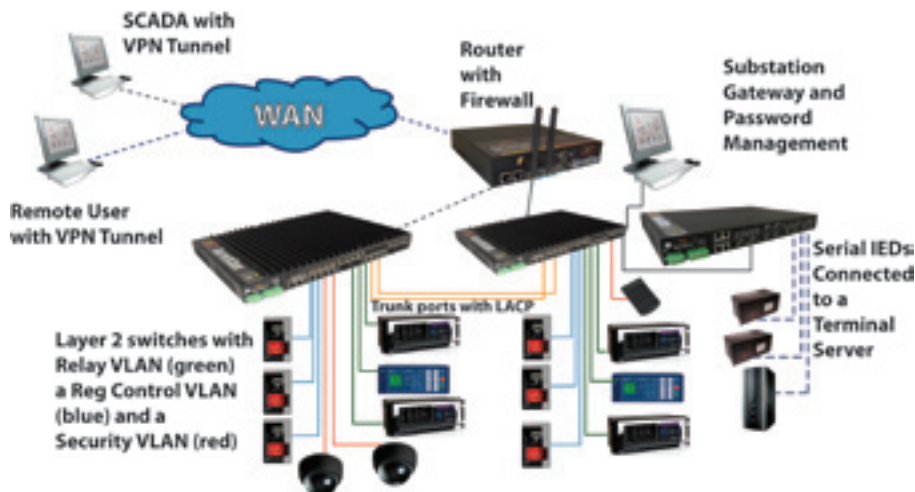
Figure 3: Typical Hybrid Substation Automation LAN with connection to WAN
