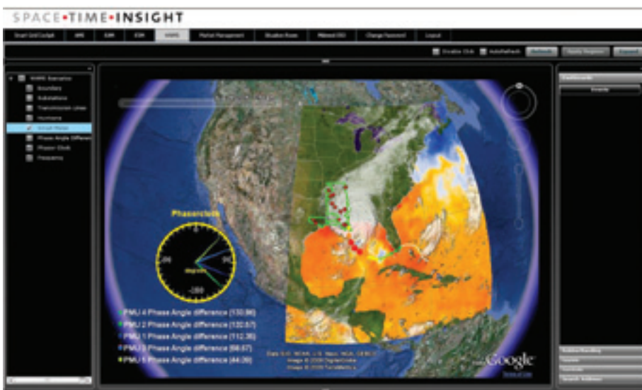
Figure 2: Space-Time Insight screenshot shows historical re-play of a hurricane over a utility's assets and the hurricane's impact on grid stability indicators for training and forensic analysis. Simulation features similarly enable scenario planning and training.
