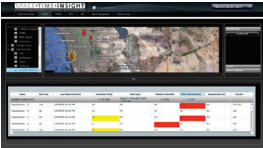
Figure 1: Screenshot of Space-Time Crisis Composite shows geospatial monitoring and alerting about fire locations, fires' relative priority status, last observed time, wind gusts and direction, relative humidity, fuel moisture levels, temperature, and proximity to critical assets and employees in the field workforce, enabling preventive mitigation and improved emergency response. Control room operators and supervisors can click to details or initiate action flows from the geospatial screen.
