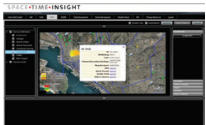
Figure 3: Screenshot of Space-Time Asset Composite shows a pop-up screen, which appears after a user has clicked on an alert within the geospatial screen. The popup offers links to preventive and remedial action scripts and workflows, work permit forms, SCADA feeds, and video footage – enabling more effective resolution of an asset-specific issue.
