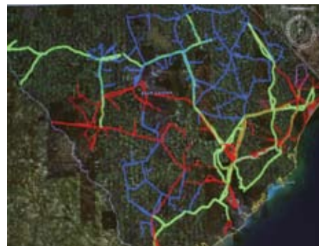
The data visualization above reflects data automatically built from GIS data and shows real-time updates from the SCADA system in KML files overlaying Google Earth.
