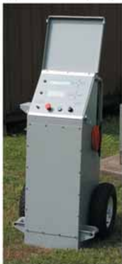
VLF Cable Testing
