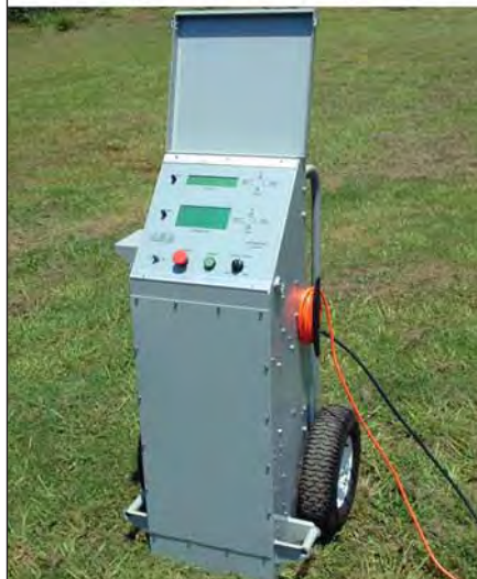
VLF Cable Testing
