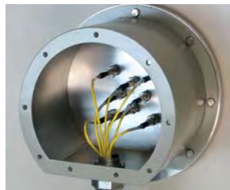
Fig. 7 Feedthrough fiber optic plate, with protection box
