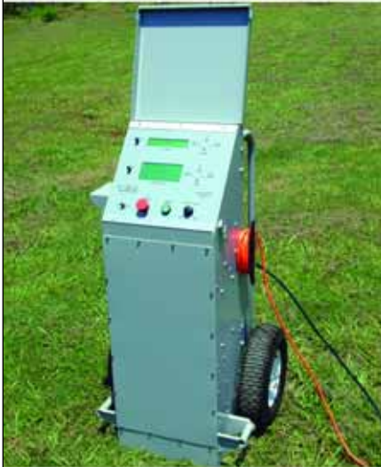
VLF Cable Testing
